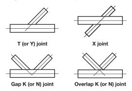
Figure 1. Typical welded joint designations
